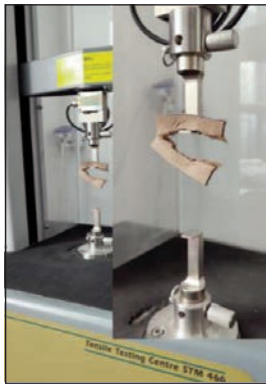
Fig. 3. Slit tear test on SATRA STM 466ST
